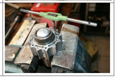
Drill the existing fixation holes on the flanges at the diameter  $\emptyset$  6.
