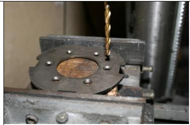
Drill a cone so that you can later put the countersunk head screws ( with  $\emptyset$  12 mm drill cut at 90° or 90° mill). Screwheads shall not be fully inserted in the flange, they shall jut out above for half 5/10 éme mm.
