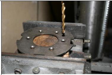
Drill a cone so that you can later put the countersunk head screws ( with  $\emptyset$  12 mm drill cut at 90° or 90° mill). Screwheads shall not be fully inserted in the flange, they shall jut out above for half 5/10 ème mm.
