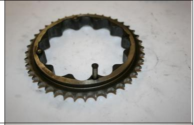
Respect the marks made during disasembly.
