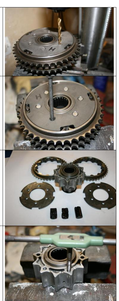
Drill the existing fixation holes on the flanges at the diameter  $\emptyset$  6.
